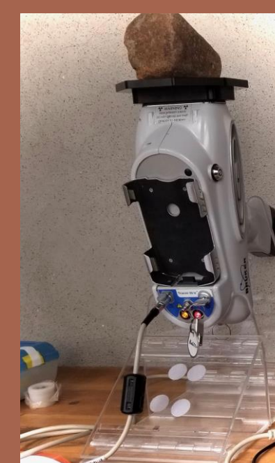
Figure 4: XRF in Benchtop mode with Loom Weight
